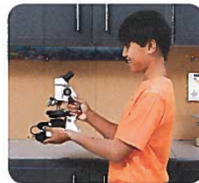
Figure 2 The microscope should be carried with one hand under the base and one hand on the arm.
